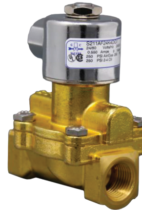
3/8", 1/2" and 3/4" NPT anti-water hammer solenoid valves in brass & nickel-plated brass body materials with stainless steel trim.
